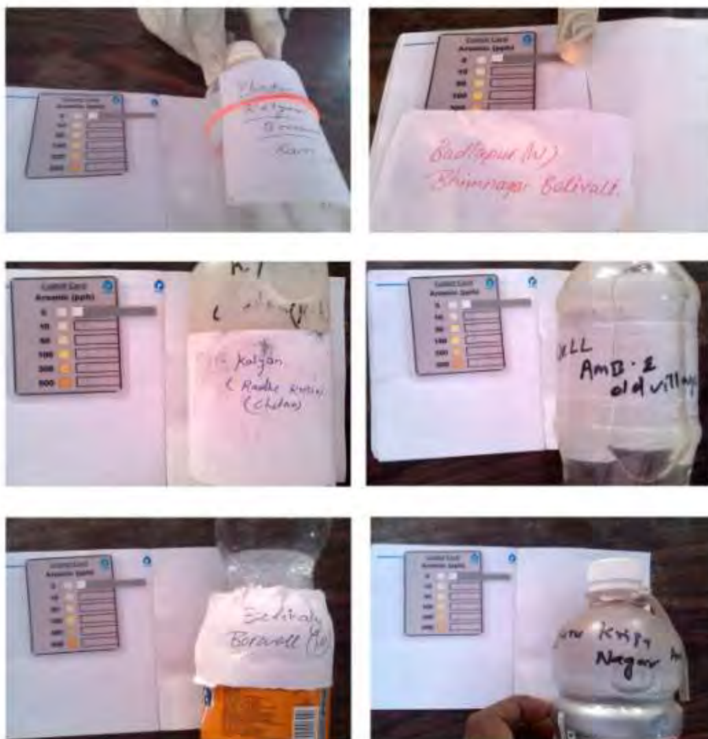
Figure 4: Photographs showing the comparison of colour change of water samples collected from various Villages/Societies with that of standard colour chart provided along with the Kit. Note that no colour change was observed indicating arsenic in these water samples is absent and if present, it is below 10 ppb (safe level as per WHO guidelines)
