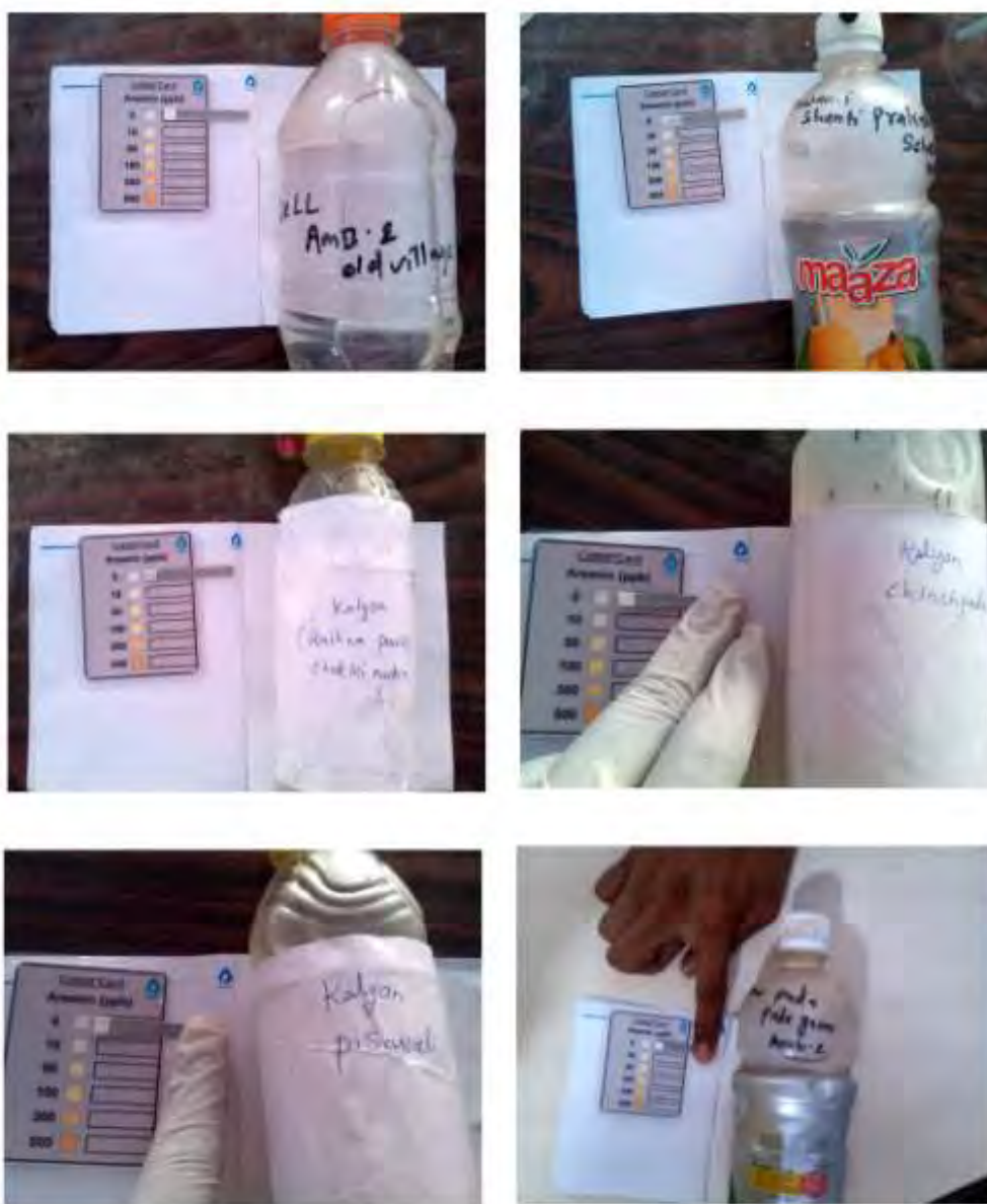
Figure 5: Photographs showing the comparison of colour change of water samples collected from various Villages/Societies with that of standard colour chart provided along with the Kit. Note that no colour change was observed indicating arsenic in these water samples is absent and if present, it is below 10 ppb (safe level as per WHO guidelines)
